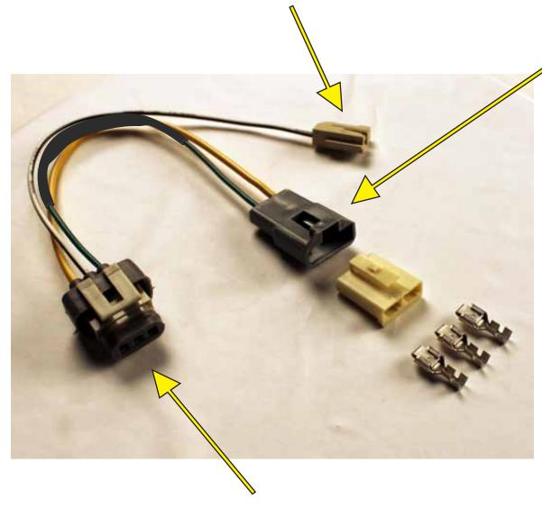
Plug this connector onto the main plug connection of the alternator.
